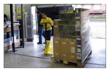
When a shipment of merchandise arrives at the store, an employee uses a pallet jack to rotate the pallet in an RFID portal's read field, to maximize the chances of reading every item.
